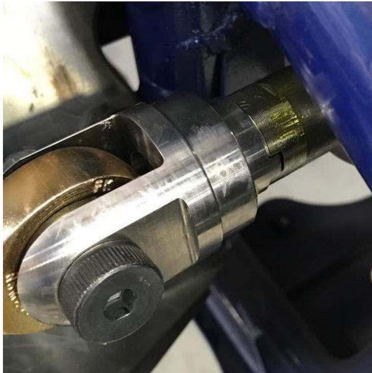
Figure 1: Install clevis onto steering box rack.
