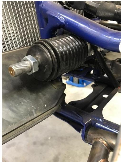
Figure 3: Steering boot installed over heim.
