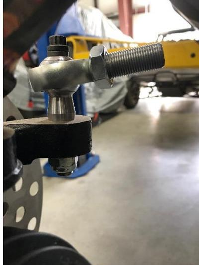
Figure 4: Tie rod end assembly.
