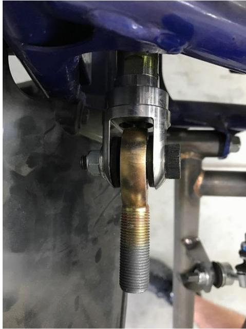
Figure 2: Install heim onto clevis.
