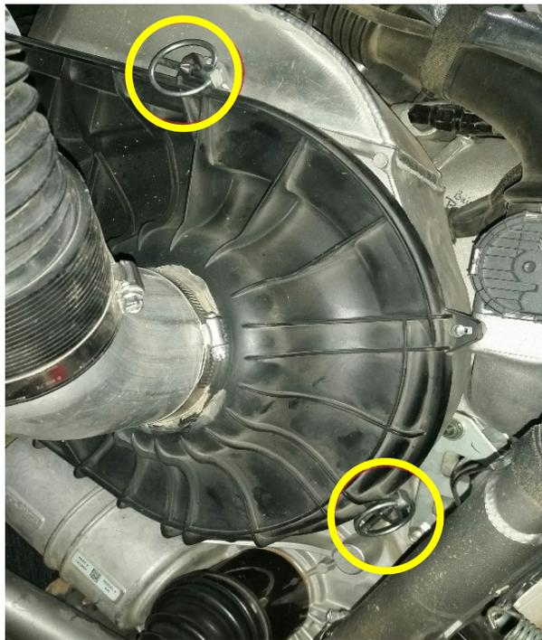
4. Finally, re-install the hose clamp and outer clutch cover as shown in figures below.
