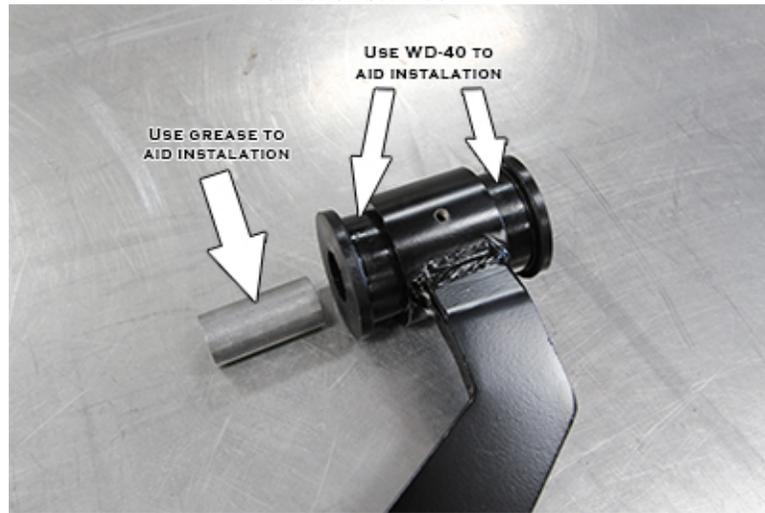
**Figure 2: bushing and crush sleeve installation**
