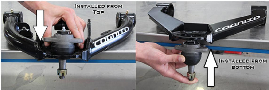
Figure 1: ball joint installation
