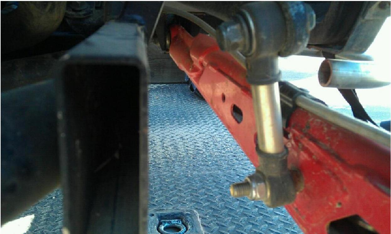
Figure 2: End Link mounted, also shown is the trailing arm gusset welded in
