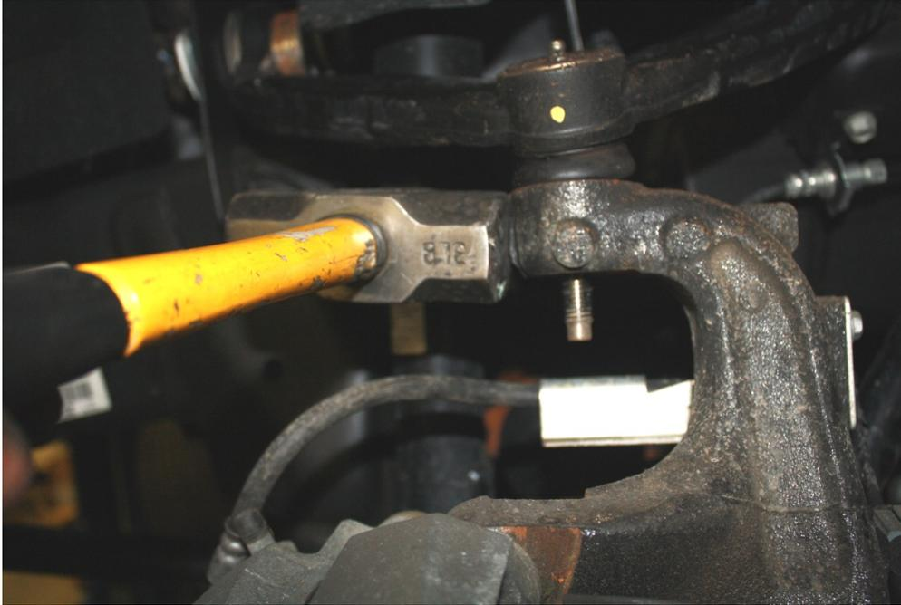
**Figure 1: breaking ball joint loose from spindle**
