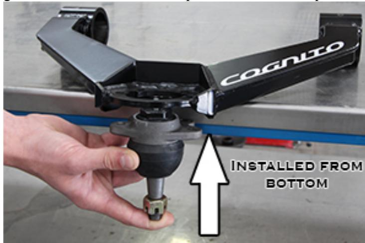
**Figure 2: ball joint installation**
