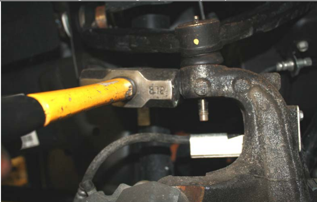
Figure 1: breaking ball joint loose from spindle
