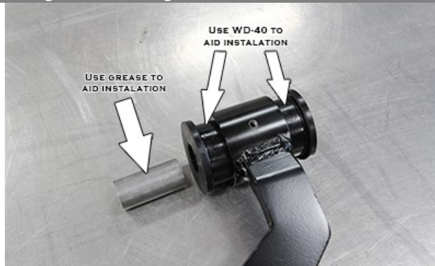
Figure 3: bushing and crush sleeve installation
