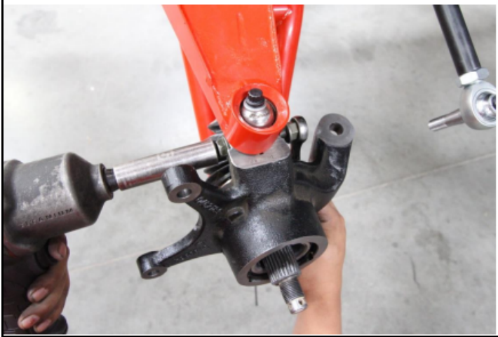
Figure 5: Tighten stud and pinch bolt.
