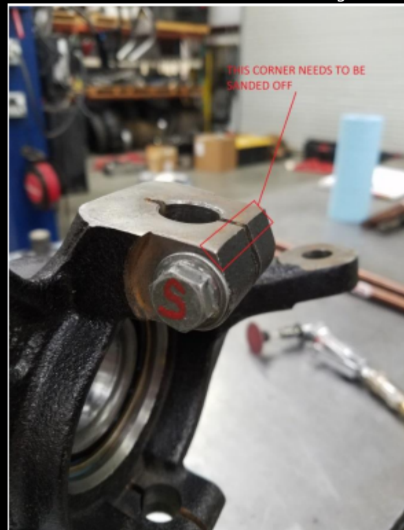
Figure 2: More detailed note of the trimming, which must be done to both areas shown in Figure 1.
