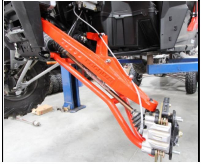
Figure 6: Brake Line Routing.
