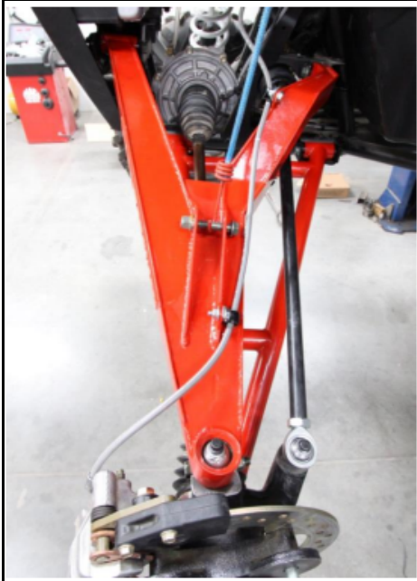
Figure 7: Fasten brake line with cushion clamps.
