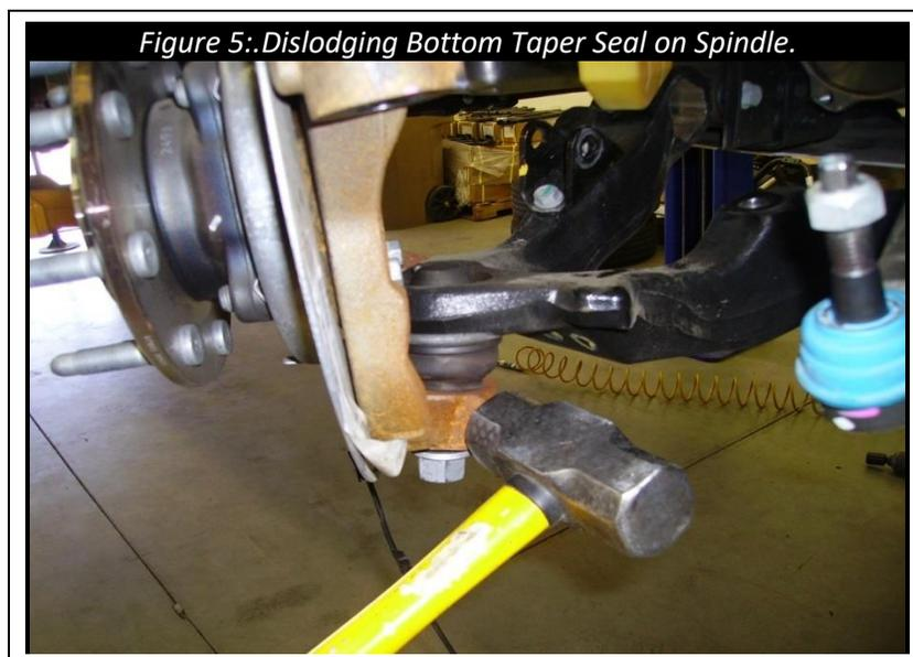
12. Next loosen the upper ball joint nut, but leave engaged by a few threads. With the spindle assembly hanging from the upper control arm, hit the spindle with a large hammer on the boss that surrounds the upper ball joint stud. This will dislodge the taper seat and free the upper control arm from the spindle. Remove the spindle assembly from the vehicle and set aside.
