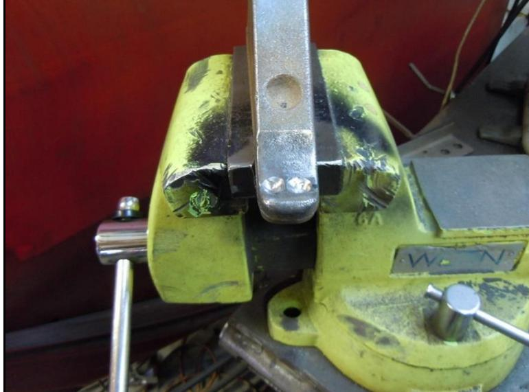
*Figure 19: Stock Torsion Key Slotted Pocket Formed.*
