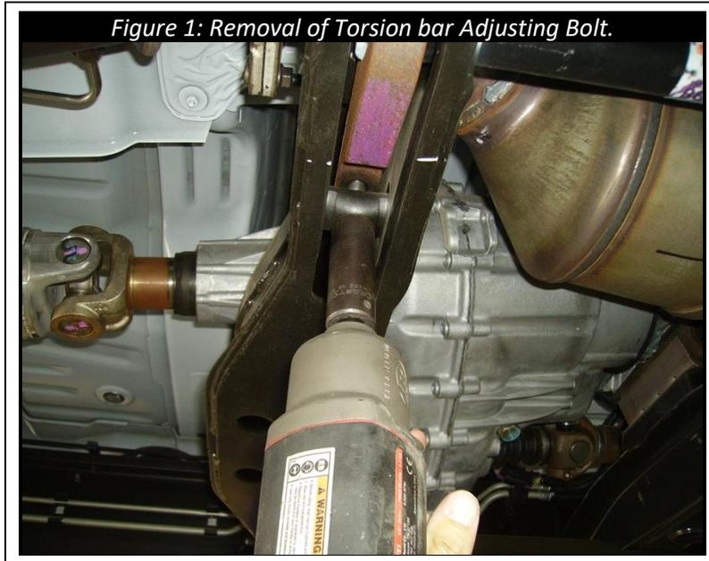
3. Slide torsion bar forward into lower control arm, this will allow the torsion bar adjuster keyway to fall out. Repeat this to the other side.
