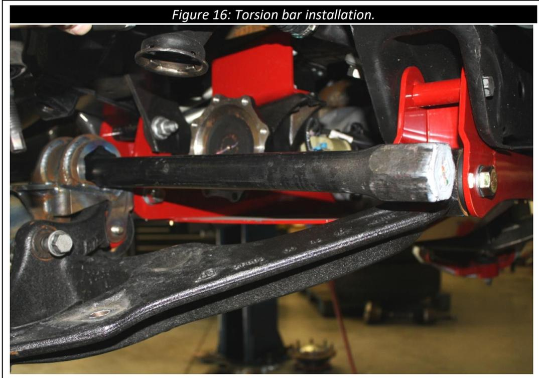
53. Install either the Cognito torsion bar keys if purchased or the OEM torsion bar keys into the torsion bar crossmember, but do not load the torsion bar.
