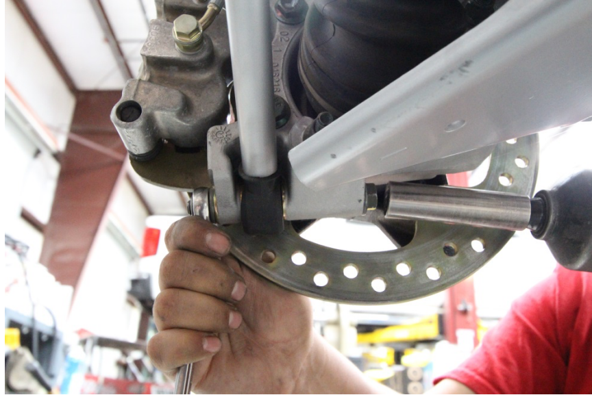
Figure 1: Remove lower radius rod from bearing carrier.
