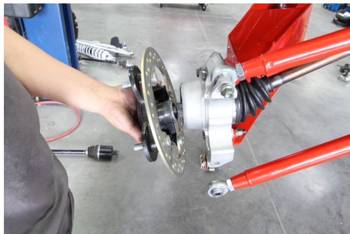
Figure 7: Install hub and rotor onto the spindle stub and in the bearing carrier.
