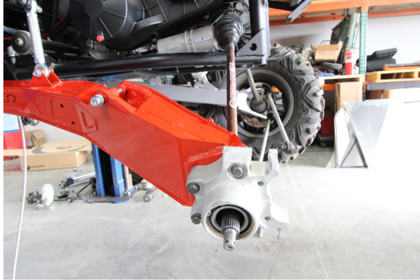
Figure 6: Insert the outer end of the axle into the bearing carrier.
