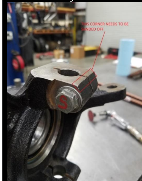
Figure 2: More Detail Shown of the Area That Needs to be Removed, Which Must be Done in Both Locations Shown in Figure 1.
